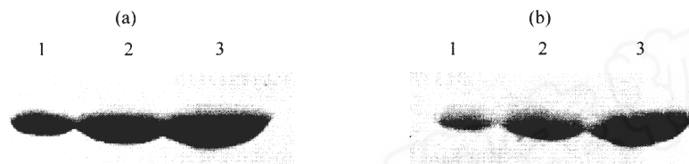
Fig.3 Current of electrophoretic transfer affected the result of Western blot (a) Current 40 mA; (b) Current 80 mA. Transfer time: 40 min, loading protein: 120 \mu g.
