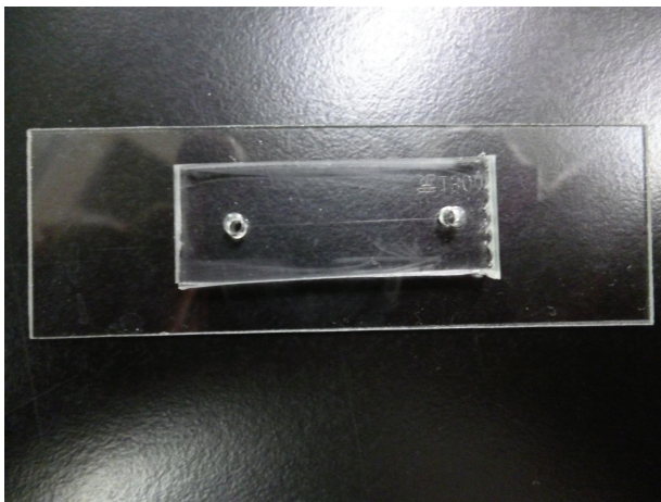
图1 用于分离的微流控芯片 Fig.1 Microfluidic chip for separation
